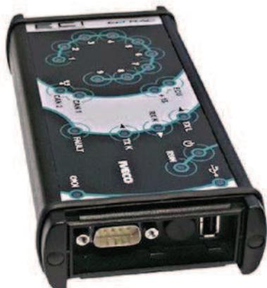
Figura 961 - Modulo ECI (Eltrac Communication Interface)
